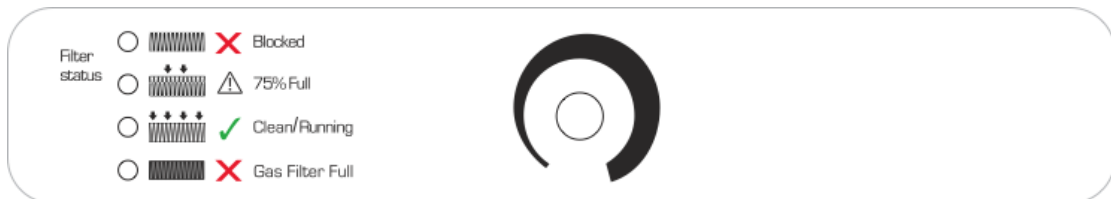
Fig 10 - Gas filter full indication - VOC monitor
